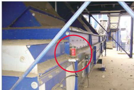
Lubrication of pillow block bearing on a conveyor
