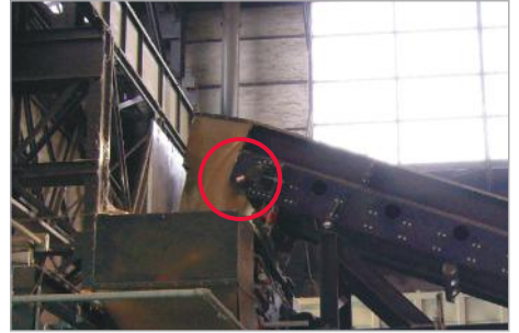
Lubrication of pillow block bearing on a conveyor
