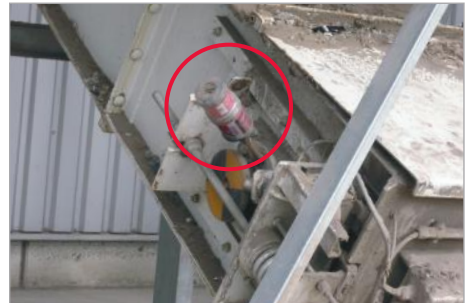
Lubrication of flange bearing
