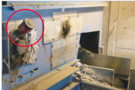
Lubrication of flange bearing on a conveyor
